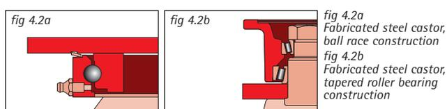
combinations of tapered roller or ball bearing races. The fork legs are usually securely welded to the swivel head forging giving an extremely strong construction suitable for heavy loads.
