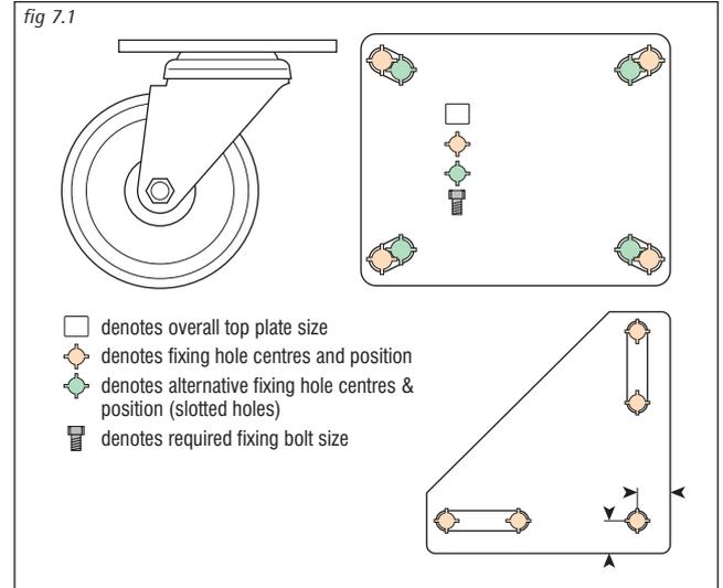
Normally a rectangular plate with four fixing holes (exceptions include 3 hole triangular plate and 2 hole rectangular plate. ISO 2184 sets out a range of standardised fixing hole centres as follows:
