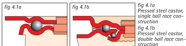
way construction. The balls run in tracks formed in the fork and top plate pressings which are secured together by a heavily riveted steel king pin.
