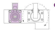
Mount truck locks as near as possible to swivel castors, without encroaching on the swivel radius. Trucks with 4 swivel castors Mount 1 truck lock at each end
